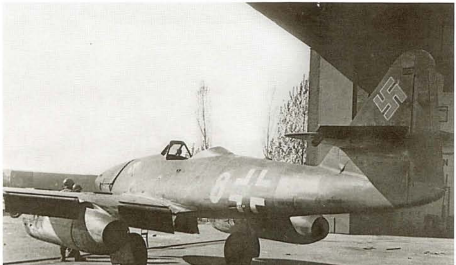
▼ 'Yellow 8,' a Leipzig-built Me 262A-1a ( Werknummer 112385), was found at Stendal-Borstel airfield in central Germany by US troops on 15 April 1945. This Me 262A-1a has a blister on the gun bay door, a feature of late production Me 262s, but lacks the broad rudder trim tab and the pilot's rear armor. It carries the badge of JG 7. Only the rear signal flare launcher is loaded, and the canopy and aft cockpit glazing have been removed. (Manfred Griebel)
