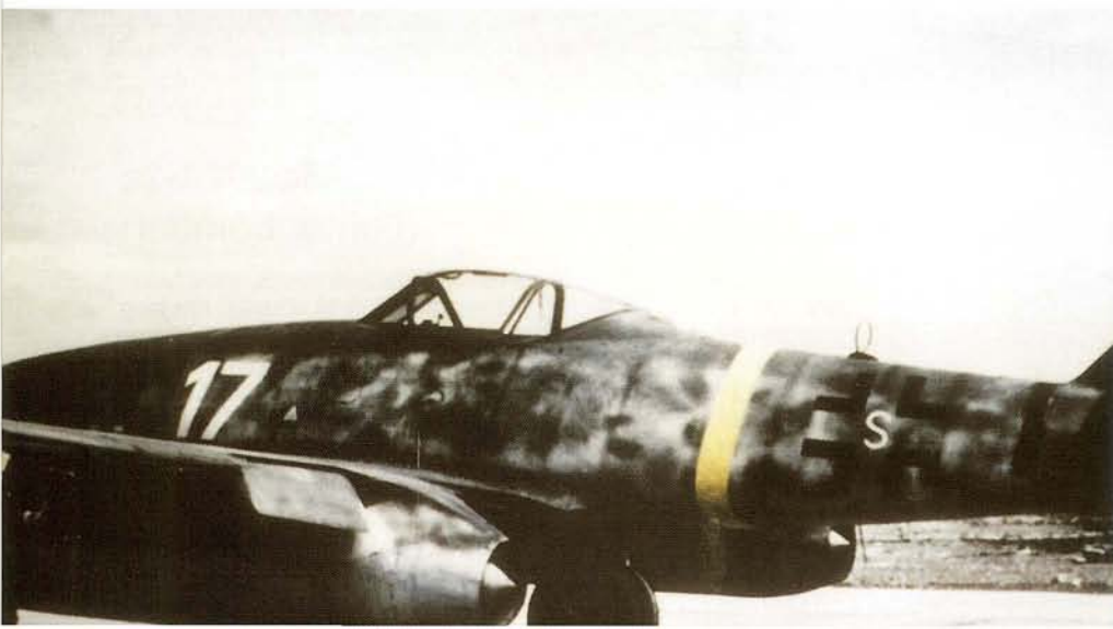
▲ This Me 262A-1a ( Werknummer 130167) first flew on 30th May 1944. It was allocated to the Messerschmitt AG for factory test trials as 'V167,' after the last three digits of its serial number, and had made over 300 flights by March 1945. In December 1944 it received a 1200 mm long nose probe for longitudinal stability tests of the airframe. (Willy Radinger)
