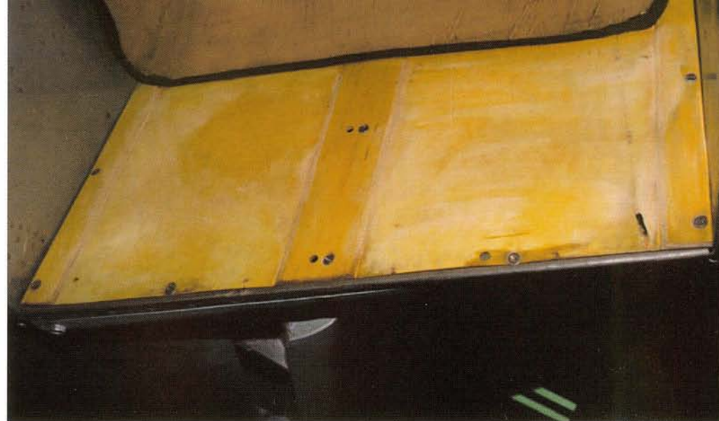
▲ Looking up into the front tank bay of 500071. The inner port wall is visible, as well as the leading edge slat in front of the port wing. The nose tank has been removed from the aircraft as well as its access panel. The tank of the Messerschmitt is also on exhibit.
