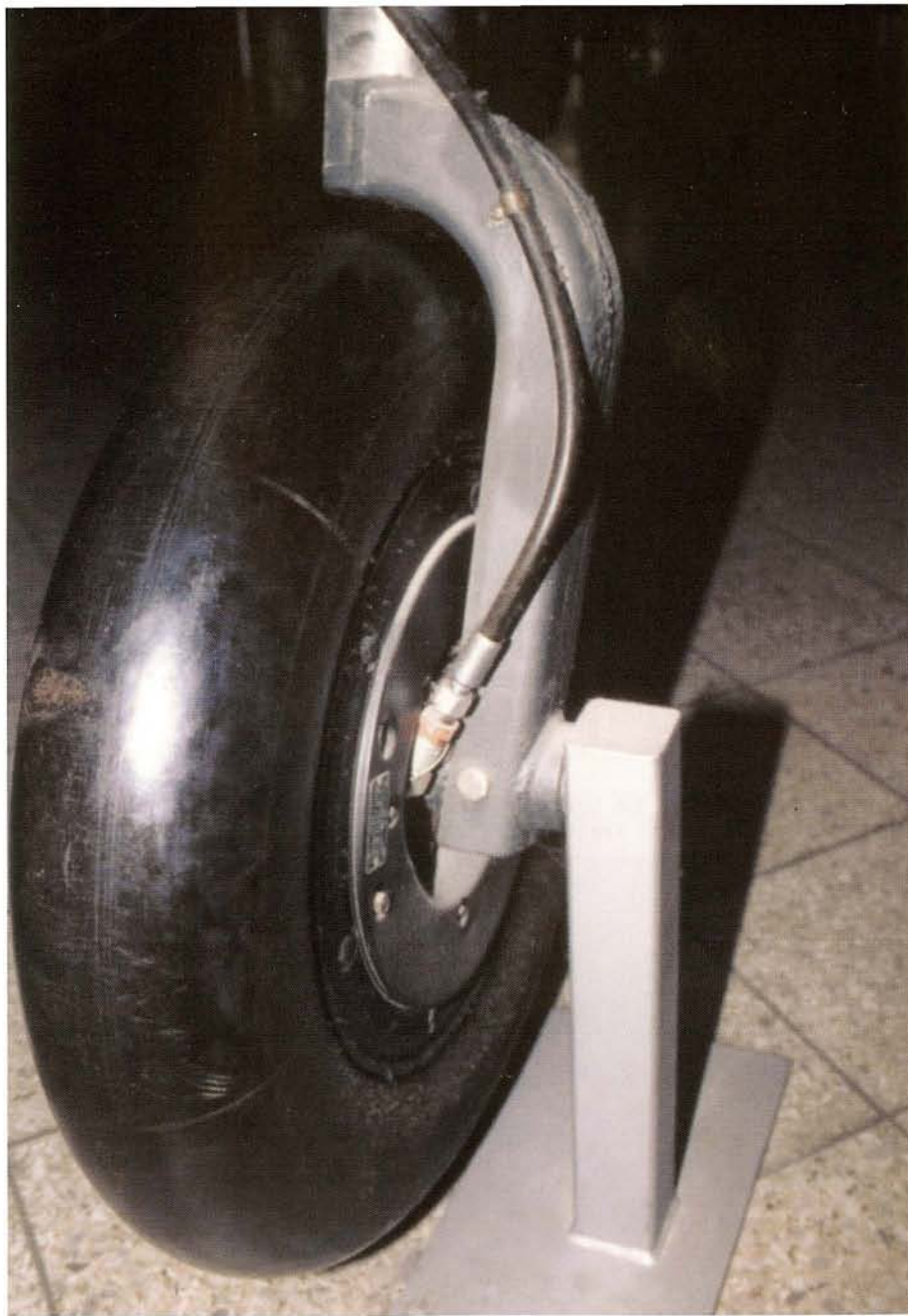
The nose gear of a Me 262A-1a consisted of a single strut. A pneumatic brake pipe was attached to the strut.
