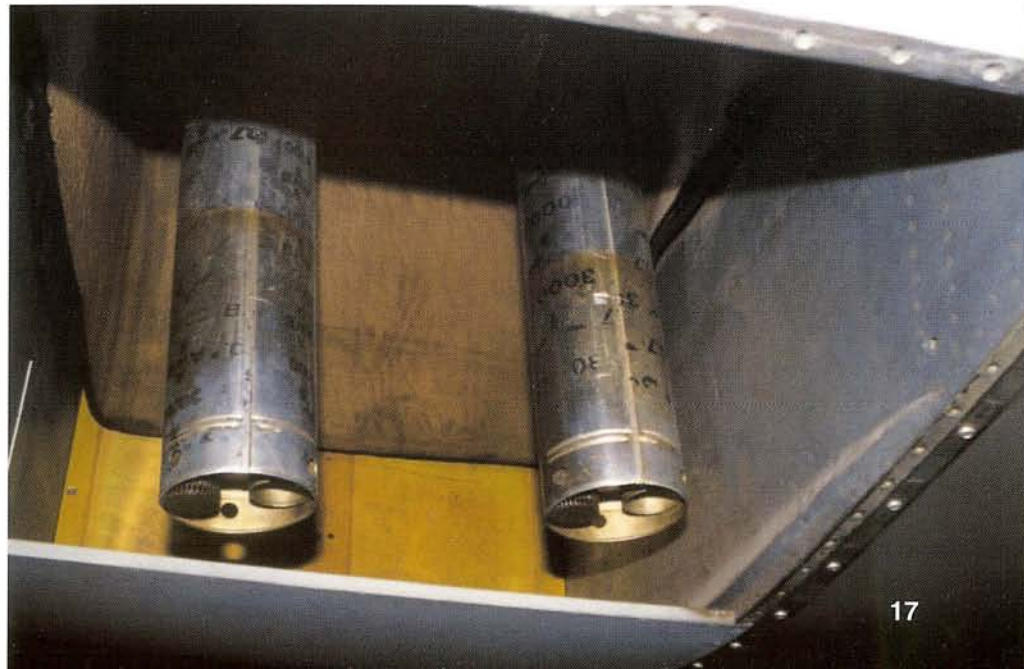
▼ Both the tank and tank cover have been removed from the lower nose, revealing the two fuel lines. The use of two identical main fuel tanks in the Me 262 made aircraft production and maintenance easier. A tank easily could be exchanged by removing the lower panel.
