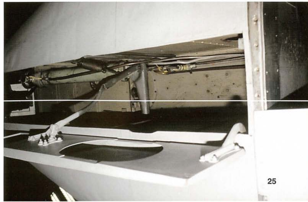
▼ The rear of the nose wheel well with the main nose wheel door mounted on the starboard side. The rear hinge is visible. The nose wheel door was attached to the fuselage by two hinges. Behind the nose wheel well is the open tank bay.
