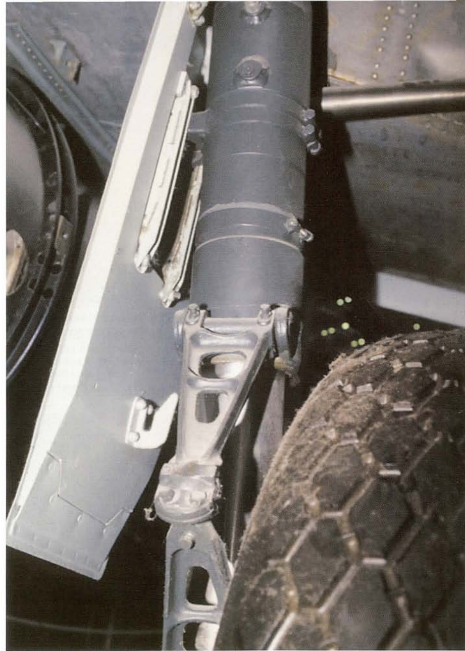
The port main landing gear of a Me 262 A-1a as viewed from the rear. The oleo scissor link as well the upper main landing gear cover door are visible.
