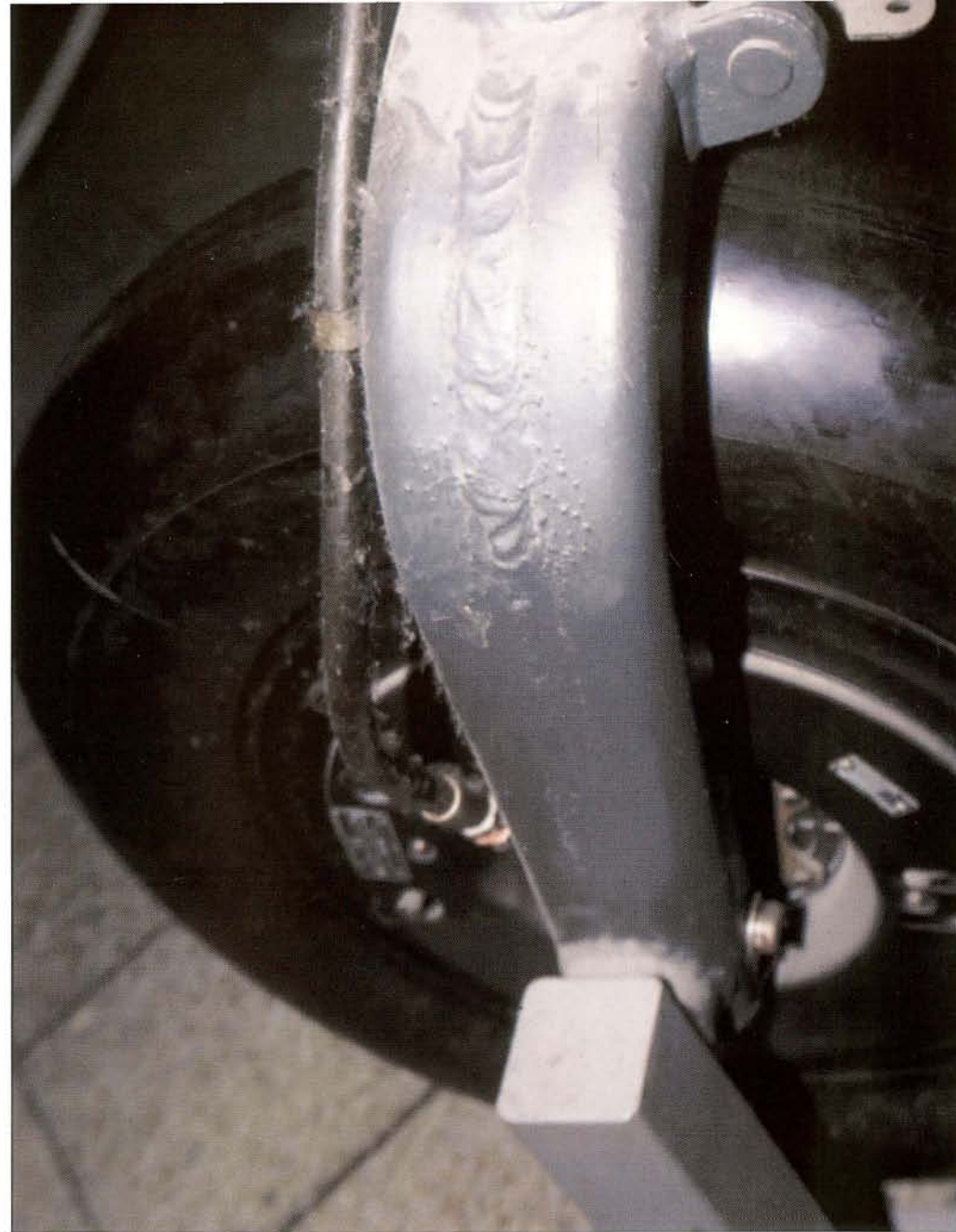
The port side of the nose wheel with the wheel strut and the pneumatic brake pipe attached to the strut.
