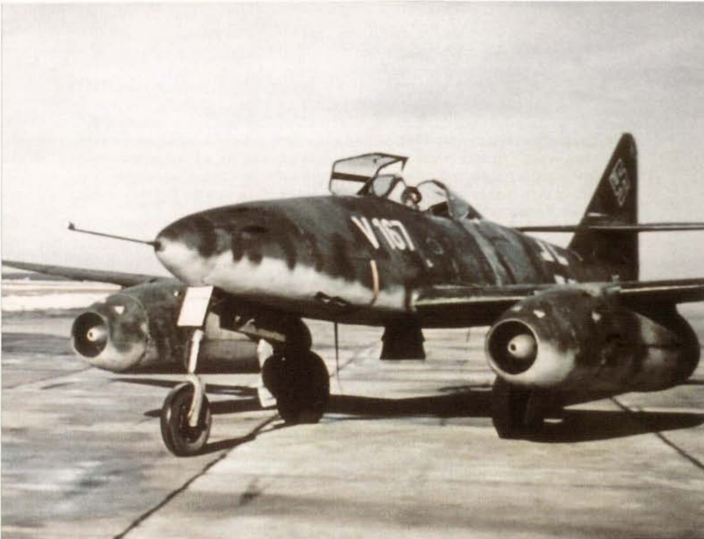
▲ This Me 262A-1a ( Werknummer 130167) first flew on 30th May 1944. It was allocated to the Messerschmitt AG for factory test trials as 'V167,' after the last three digits of its serial number, and had made over 300 flights by March 1945. In December 1944 it received a 1200 mm long nose probe for longitudinal stability tests of the airframe. (Willy Radinger)
