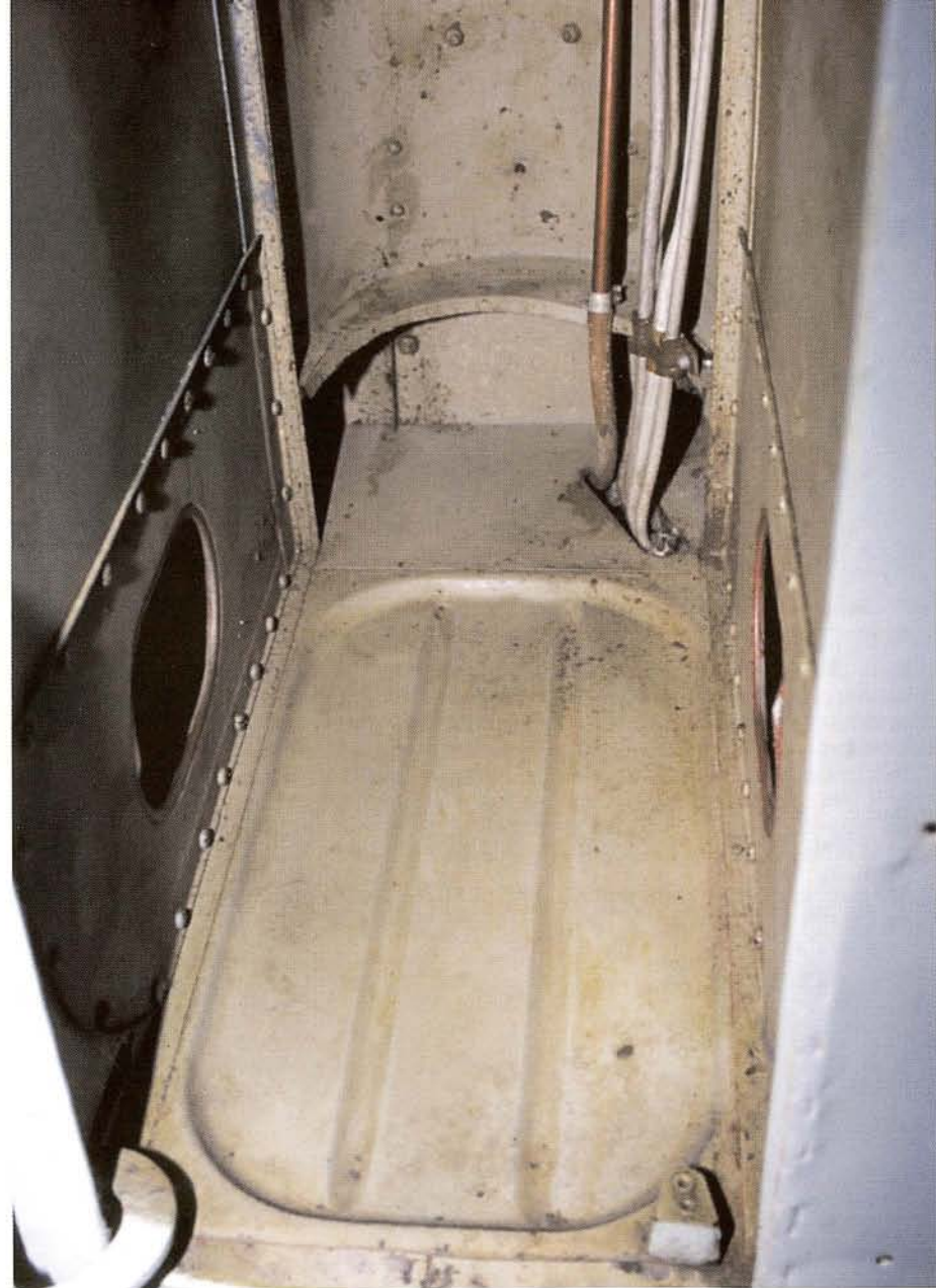
▲ Looking aft into the nose wheel well of 500071. Electrical wiring is visible at the top.
