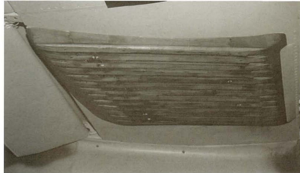
▲ The starboard EG-R4M wooden launching platform. The platform was attached to the wing with four screws, and U-shaped launch rails were fixed into the slots. It was not painted but impregnated with a liquid preservative. The EG-R4M platform was a field modification.
