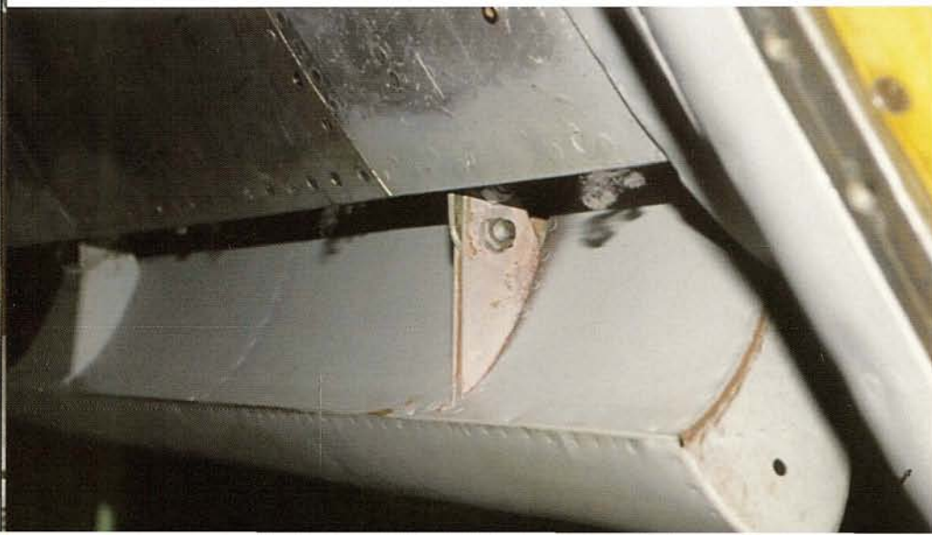
▼ The port inner leading edge slat of a Me 262 as viewed from below. The hinges were heavier than those of the outer two slats because of the heavier weight of the inner slat.
