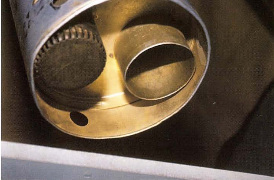
▲ A fuel filter was attached to the bottom of each fuel feed pipe.
