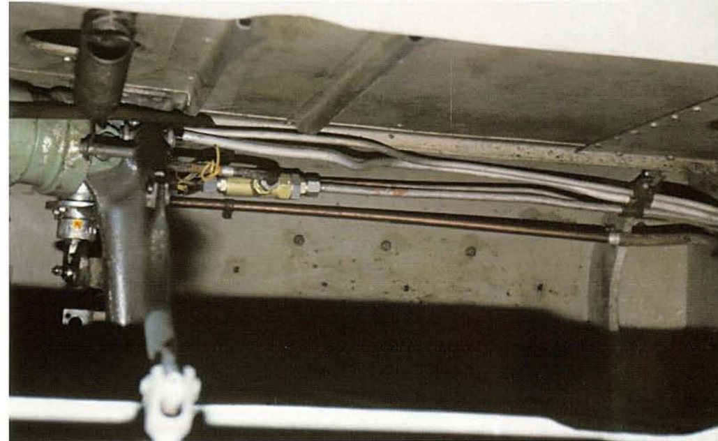
▲ The electrical and pneumatic wiring in the nose wheel well of 500071.
