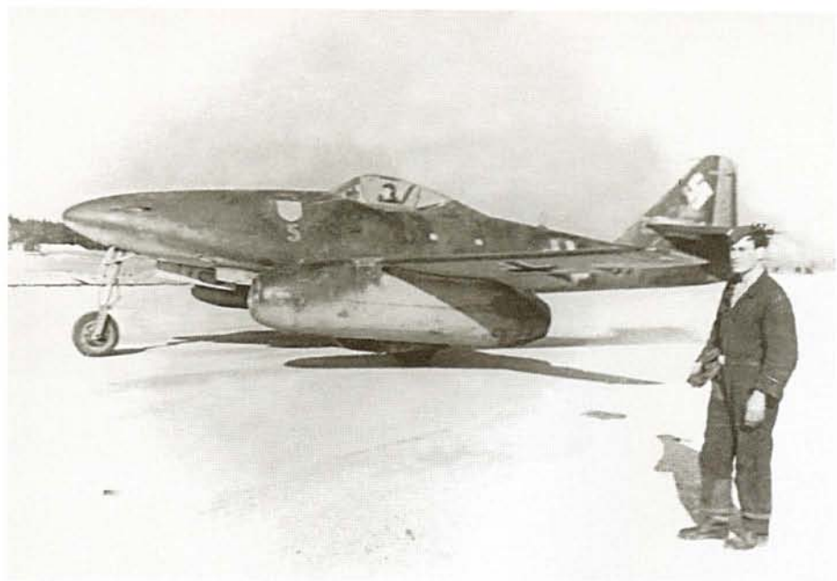
▲ An Me262A-2a of Kampfgeschwader 51 prepares for takeoff. The unit marking is painted above the letter 'S,' which stood for Schule (training). The white Hakenkreuz (swastika) is non-standard. The upper two cannons have been deleted and the upper gun port faired over. The ETC 503 bomb rack is visible on the lower nose surface. (Martin Kyburz)
