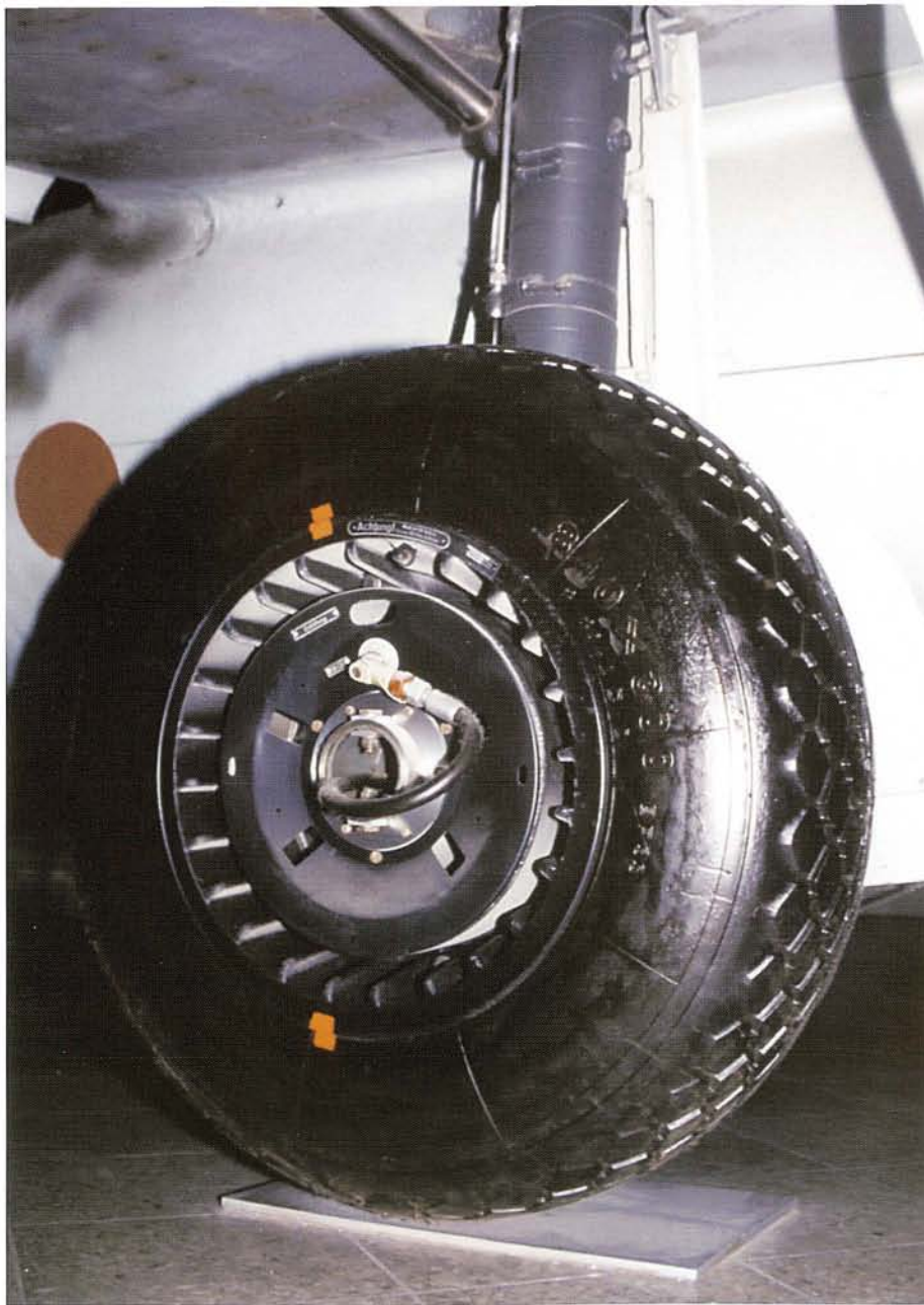
The starboard main landing gear. The main landing gear legs were manufactured by the Adam Opel AG , a subsidiary of the American General Motors company, at Rüsselsheim, Germany.
