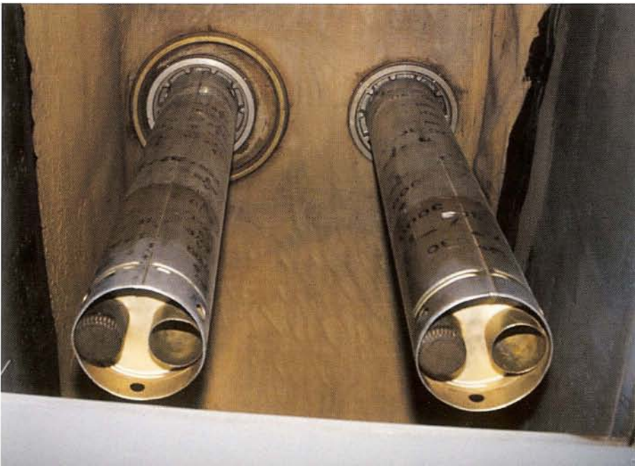
▼ The two pipes lead to the fuel pumps in the tank. Below is visible the nose wall of the front fuel tank bay.
