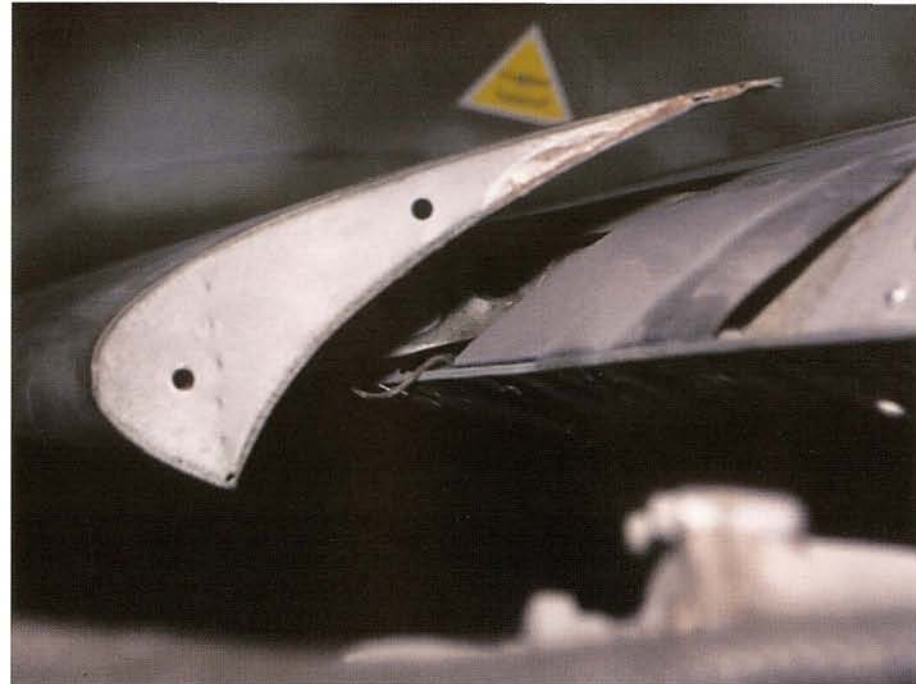
▲ The outboard end of the inner leading edge slat, adjacent to the engine nacelle, reveals its cross-section. These parts were built by the Arwa Strumpfwerke at Auerbach, a plant which formerly produced hosiery for the private consumer before World War II.
