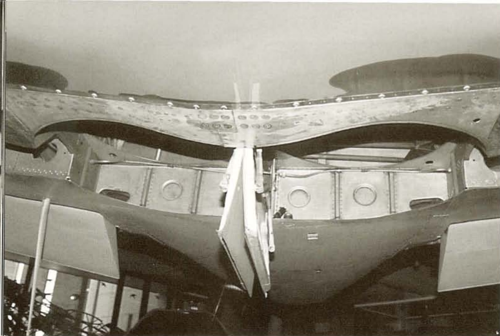
▲ Looking aft into the main wheel wells of 500071. Behind the starboard main wheel well is the antenna for the Lorenz FuG-16ZY radio. The four circular cutouts are found only in the rear wall of the main wheel wells.
