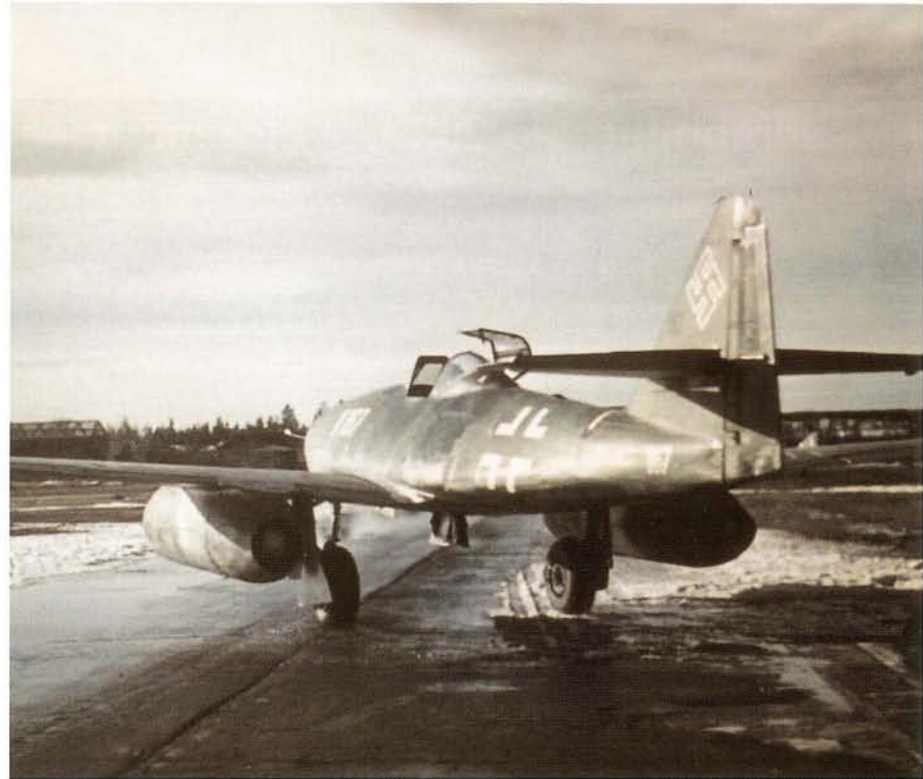
▲ 'V167' was involved in a wide variety of tests. This particular Me 262A-1a was assembled by the Autobedarf Schwäbisch Hall at Schwäbisch Hall-Hessental airfield, a subsidiary of Messerschmitt AG Augsburg. A typical feature for Schwäbisch Hall-built Me 262s was the lack of rearming instruction placards for the MK-108 cannons below the gun bay doors. Me 262s assembled at the Autobedarf Schwäbisch Hall had only the last three digits of the Werknummer (factory number) painted on both sides of the tail. Schwäbisch Hall-Hessental continued with this practice until production came to a halt in late March 1945. (Willy Radinger)
