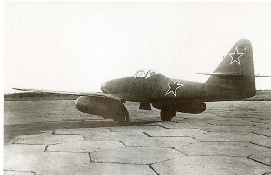
▲ The Soviet Me 262A-1a lacked the Peilrahmen (direction finding antenna) PR-16 for the Zielflug-Verstärker ZVG-16 homing amplifier, which was connected with the Lorenz FuG-16 ZY radio. The Soviet national markings were applied on the wing undersurfaces as well as to the rear fuselage and tail fin. No national markings were applied on the upper wing surfaces, which was common for Soviet Air Force aircraft during World War II. The red star was outlined with a wide white and narrow red border. (G.F. Petrov)
