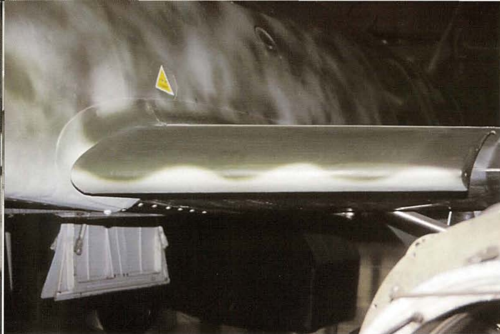
▲ The leading edge slat of the Me 262A-1a was comprised of three independent sections. A single slat was attached to the wing leading edge between fuselage and engine nacelle. The slat shown here is fully deployed. This was the standard setting for takeoff or landing.
