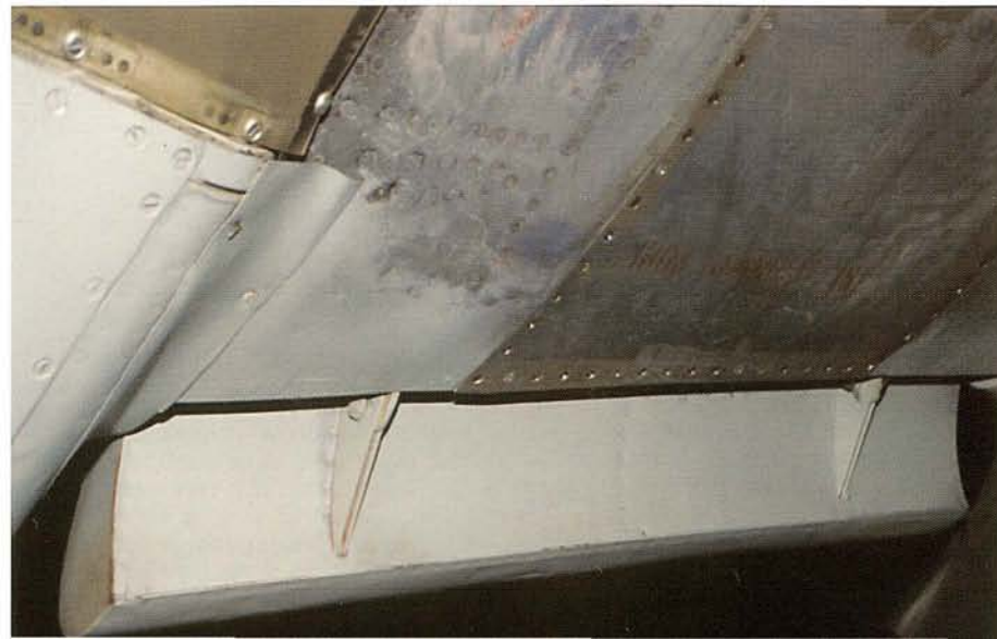
▼ The starboard inner leading edge slat of a Me 262. Each slat was attached by two hinges to the wing leading edge. The slats were operated hydraulically.
