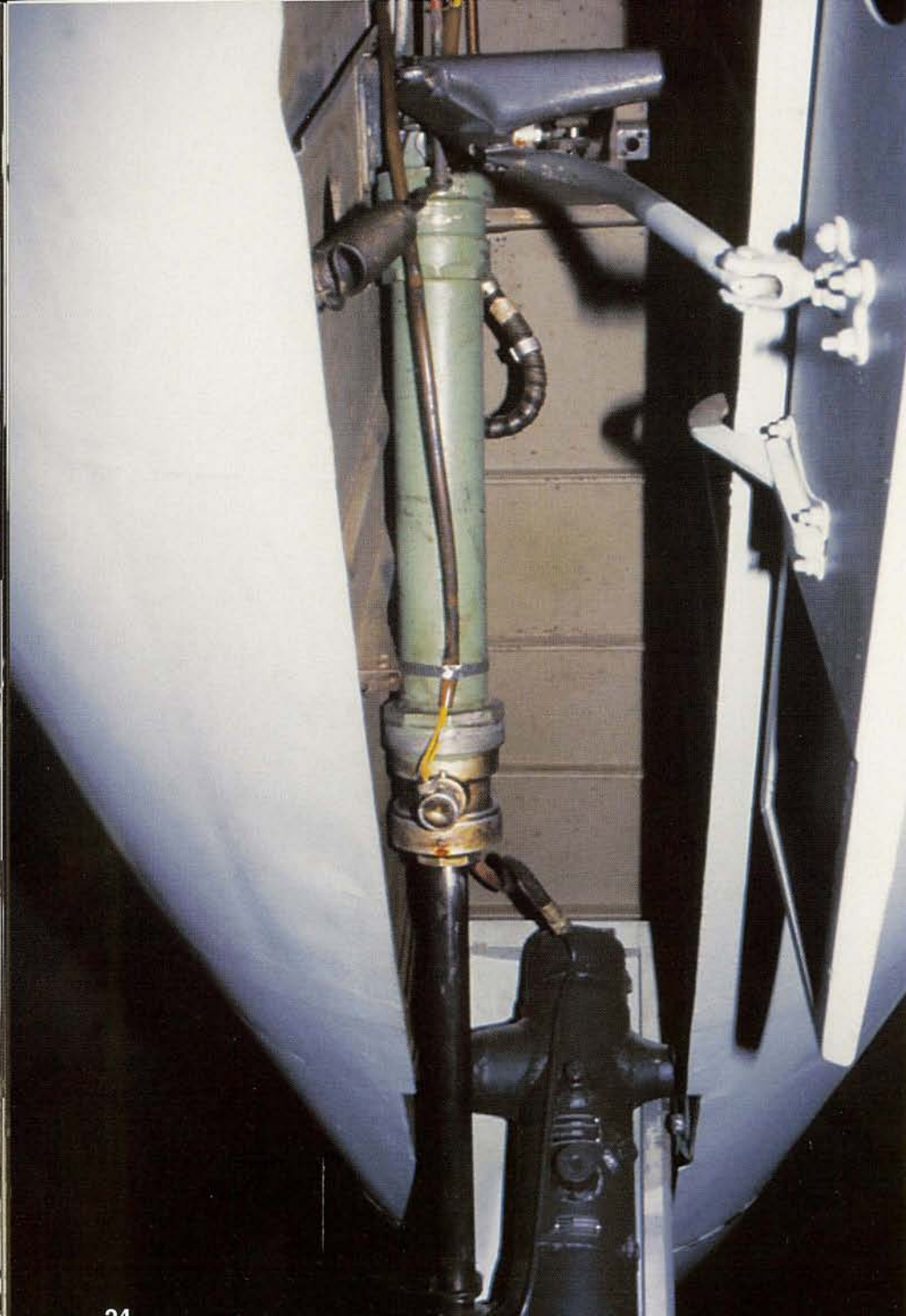
▲ Looking aft into the nose wheel well of 500071. Electrical wiring is visible at the top.
